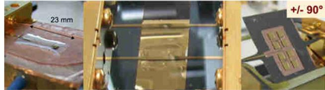
mm-wave devices on soft polymer membrane, from left to right pneumatic tunable patch antenna, phase shifter, beam steering antenna.
