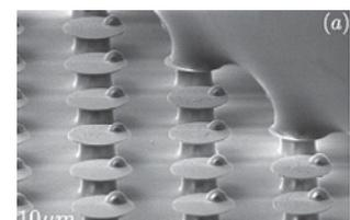
SEM images of droplet on an inclined omniphobic surface.
