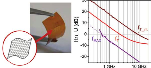
Graphene FET on kapton using solution-based graphene monolayer, and measured HF performance
