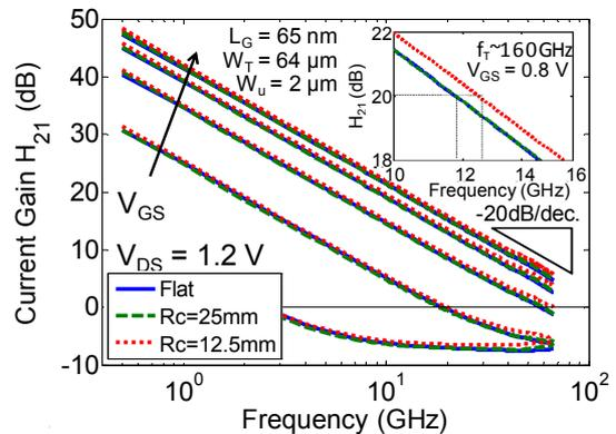
HF characteristics of UTB n-MOSFETs under flexure: using neutral plane engineering the unity current gain cut-off frequency ( $f_T$ ) is weakly impacted by strain.
