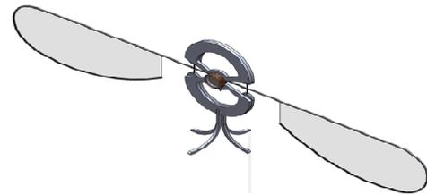
Design of OVMI prototype fabricated with SU-8
