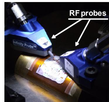
Flexible a UTB chip under HF probing in bent configuration. Same methodology was used SOI-CMOS, AllnAs/GalnAs and GaN HEMT.
